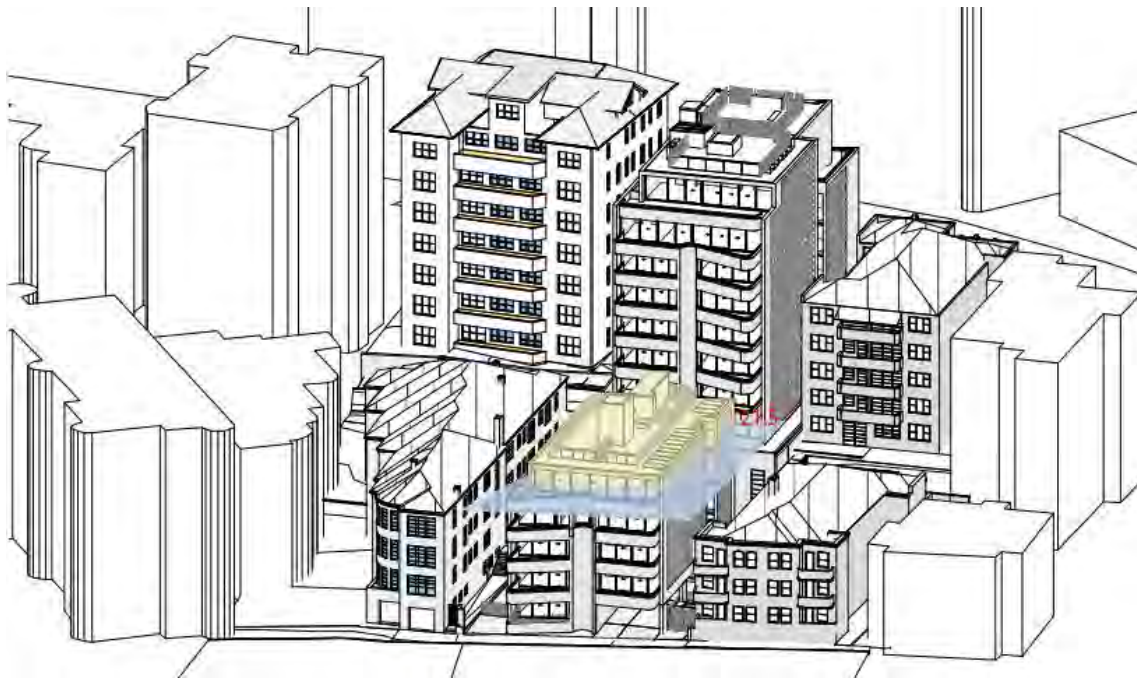
Figure 6: Mark up of the sun eye view diagram demonstrating the accurate portion of building that sits above the building height limit as highlighted in yellow.
