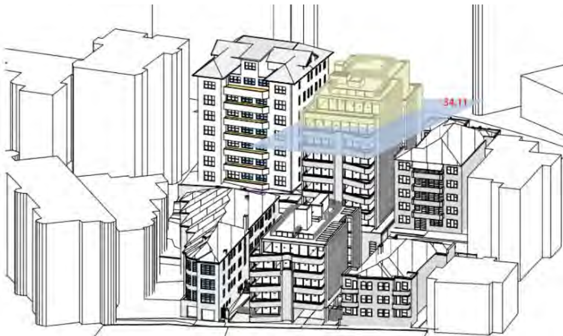
Figure 5: Mark up of the sun eye view diagram demonstrating the accurate portion of building that sits above the building height limit as highlighted in yellow.
